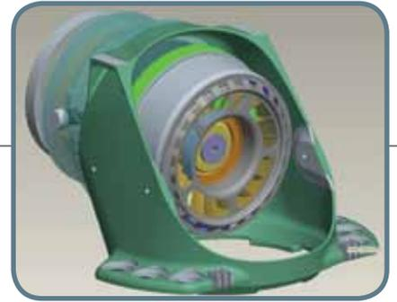
The medium speed, permanent-magnet generator, dubbed **MegaFlux**, is rated for 10.6 MW. The unit is 98.3% efficient, a 1% improvement over the Liberty and 2 to 4% over conventional induction generators. The medium speed will generate fewer natural frequencies to dampen compared to the company's Liberty quad generator. Multiple independent output windings per generator provide the same quad redundancy in the electrical system as the Liberty design.
